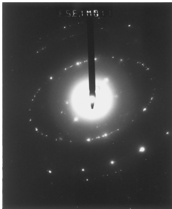
Figure 2 Electron diffraction pattern of ball-milled h-BN powder: elliptic rings characteristic of a "turbostratic" material. The first intense elliptic ring relates to the (00.2) crystallographic plane.
